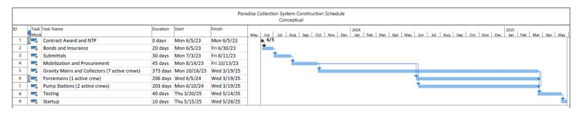
Figure 3. Estimated Collection System Construction Schedule
