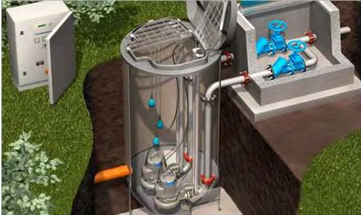
Figure 30 Wet Well Diagram
