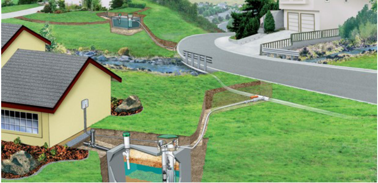
Figure 5.3 – STEP and STEG Collection Systems
