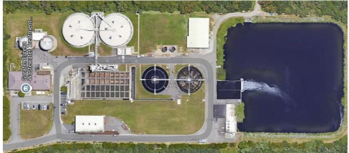
Biotrickling filters (top, white circles), clarifiers, and effluent storage (right) [Solids pond and ocean outfall not shown]
