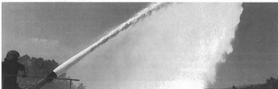
Figure 18 Firefighting Water Cannon Using Surfactant Foam
