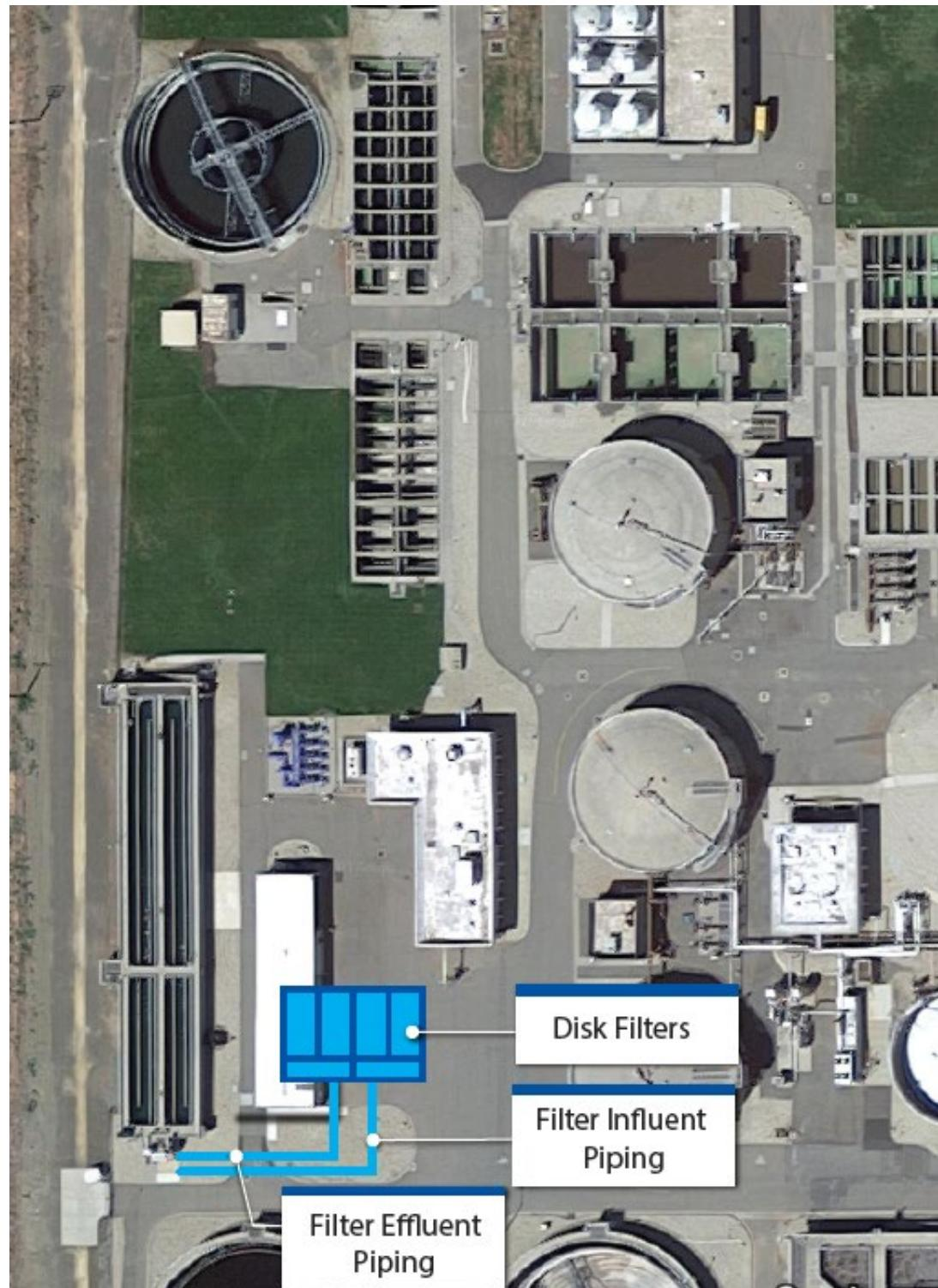
Figure 5.4 Potential Layout for Disk Filter Facilities at WPCP
