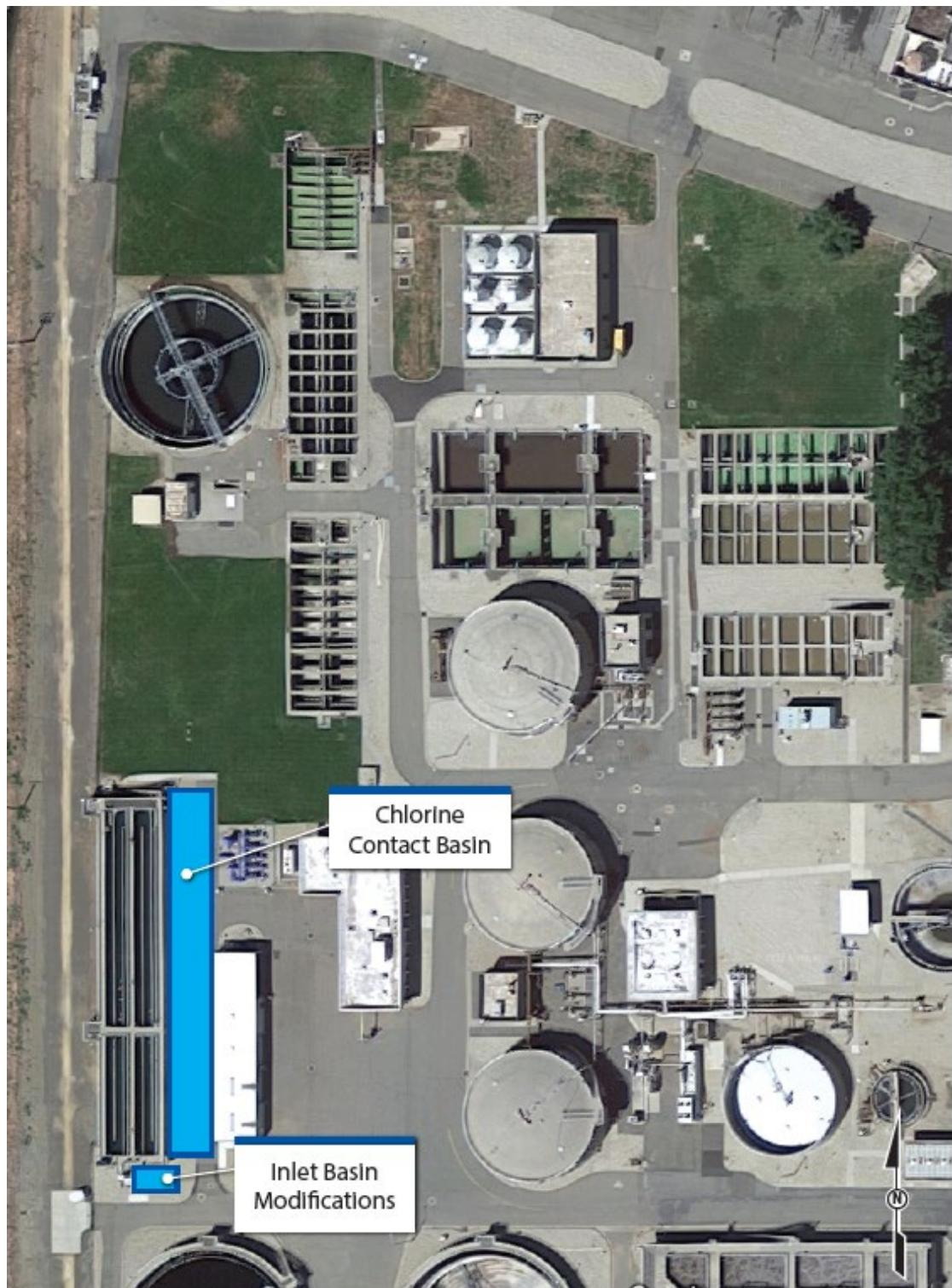
Figure 4.6 Chlorine Contact Basin
