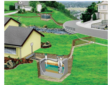
STEP collection (Photo courtesy of Orenco Systems)
