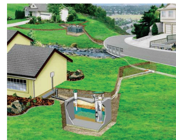
STEP collection (Photo courtesy of Orenco Systems)
